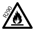
Flammable material. This appliance contains R290/Propane a flammable refrigerant. Refer to this manual for safety information.R290 refrigerant gas complies with European environmental directives. Do not pierce or burn. Maintenance and repairs requiring the assistance of other qualified personnel must be carried out under the supervision of specialists in the use of inflammable refrigerants.
