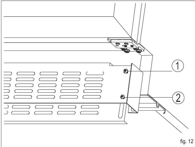
1. Remove the screws (1) from both the top left and top right hand sides.
