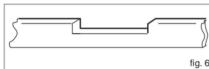
This appliance is designed to fit under worktops between 820 – 890mm in height, using the adjustable plinth plate to ensure that the feet are concealed from view.
