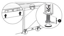
The adjustments work identically for both front levelling feet.
