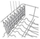
2 Locate assembly slot **1** on cup rack and firmly pop rack off support bar on that side.
