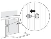
**2** Drive a wood screw (Φ 4.5 x 12 mm) through the mounting bracket and into the cabinet frame.
